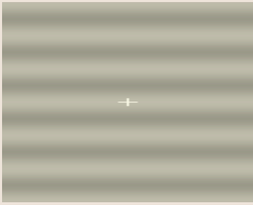
Sinusoidal grating - visual stimulus used for sweep VEP testing
